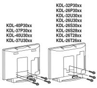
If using an electric screwdriver, set the tightening torque at approximately 2 N·m (20 kgf·cm)
